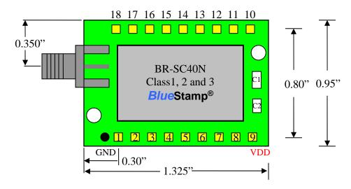
External power supply decoupling capacitors C1 and C2 are optional. C1 = 10uf Capacitor, 0805 Ceramic C2 = 0.1uf Capacitor, 0603 Ceramic
